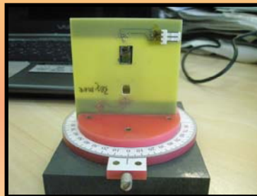
Photo of the experimental set-up used for receiver measurements
